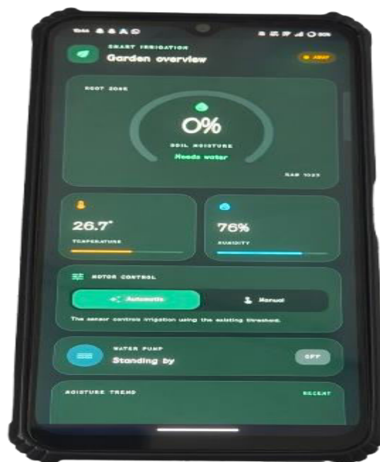
Fig.4. Real-time sensor data from the proposed IoT-enabled drip irrigation system.
